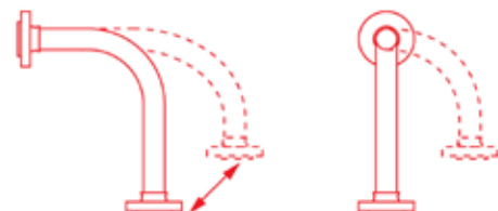
INCORRECT - Flexing movement takes place in 3 dimensions so torque is applied
